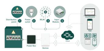
4 Or, use the Smappee Input Module to count pulses of sensors, meters and other devices or to monitor state changes (low/high) to trigger other processes.
